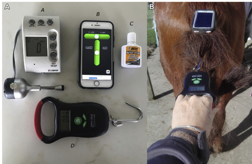
Fig. 2. Equipment needed and technique used to perform the study. 2a) Equipment used: the JTECH Commander pressure algometer (A), clinical bubble level app (B), 'Wite-Out' correction fluid (C), and digital fish scale (D). 2b) Example of caudal traction setup.
